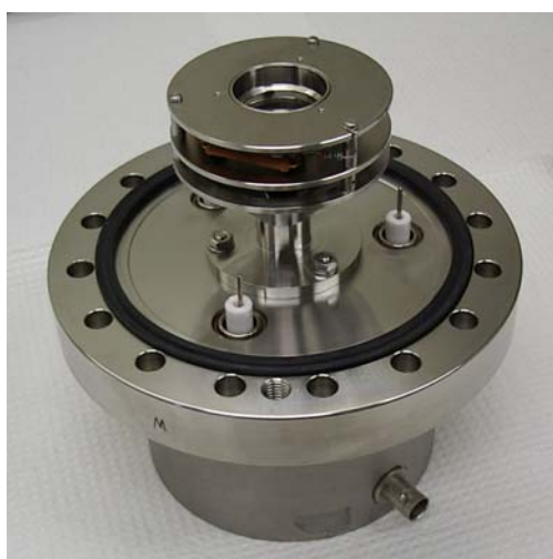
Fig. 3-19 Microchannel plate detector mounted on a flange, and circuit of it.
