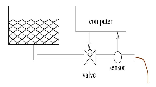
Flow to remain constant. Sensor measuring flow. Opening and closing of valve takes 10 secs (special case of an **actor**).
