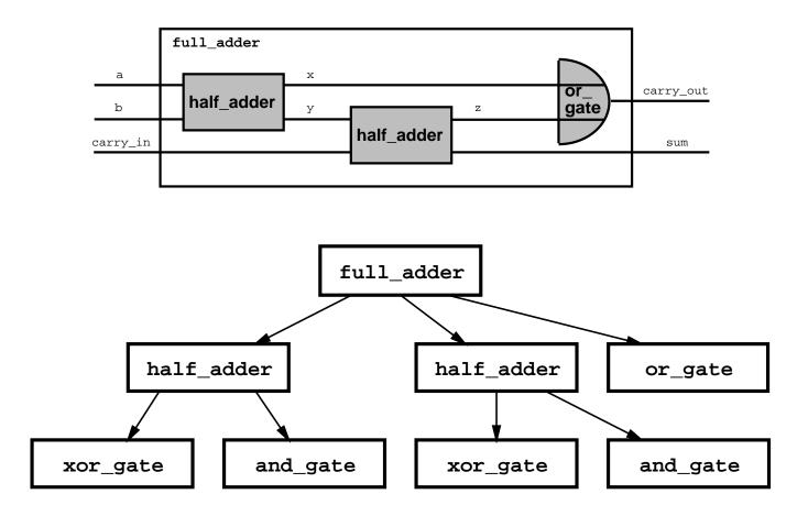
ARCHITECTURE structure OF full\_adder IS COMPONENT half\_adder PORT (i1, i2:IN Bit; carry:OUT Bit; sum:OUT Bit); END component; COMPONENT or\_gate PORT (i1, i2:IN Bit; o:OUT Bit); END component; SIGNAL x, y, z: Bit; BEGIN s1: half\_adder PORT MAP (a, b, x, y); s2: half\_adder PORT MAP (y, carry\_in, z, sum); s3: or\_gate PORT MAP (x, z, carry\_out);
