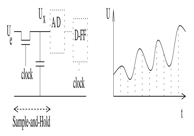
Ideal case: width of clock signal = 0, full signal amplitude available at output
