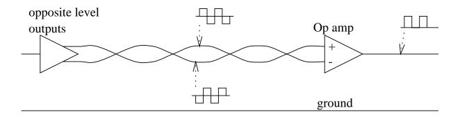
Used in combination with twisted pairs. Most noise added to both wires.
