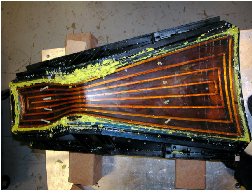
Figure 7: Photograph of the coil used to reshape the full-sized liner.
