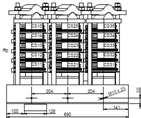
Figure 13: Design drawing of 260kA 15kVdc thyristor module
