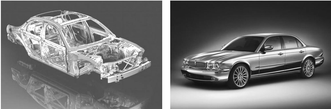
Figure 2: Self-supporting aluminum car body in Jaguar XJ [3]
