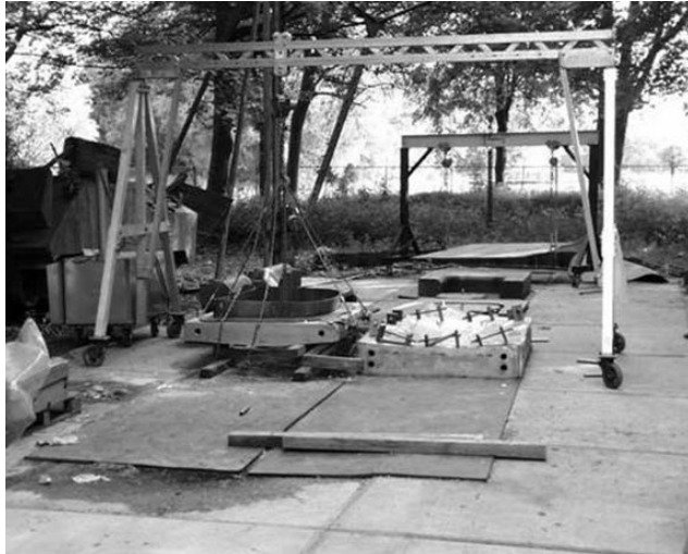
Figure 6: Stationary pool for explosion forming
