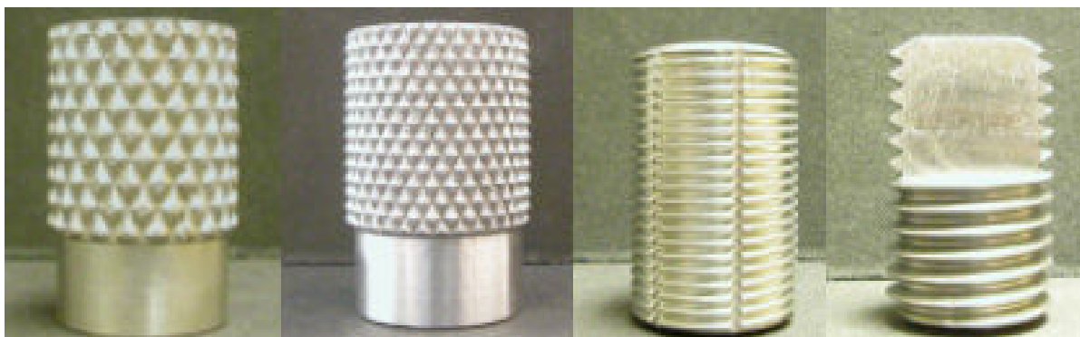
Figure 4: Example of some of the mandrel surfaces. Left to right: coarse knurl, fine knurl, fine screw thread with axial grooves, and coarse screw thread
