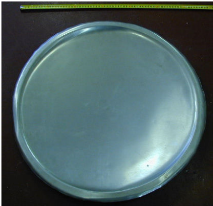
Figure 5: Forming of 600 mm Al Antenna Disc
