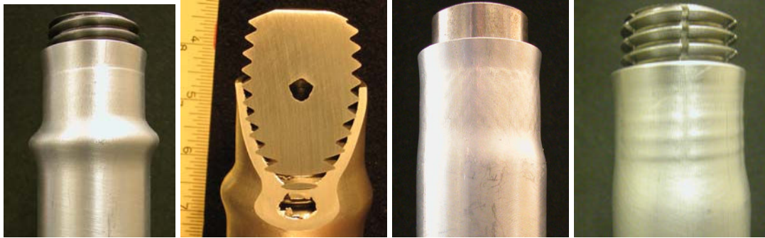
Figure 5: Examples of crimp joints based on surface impression. From left: joint based on a 25.4 mm coarse screw thread tested in compression (14 kJ impulse onto a coarse thread screw); angled cross section of similar joint; a joint based on a knurled mandrel
