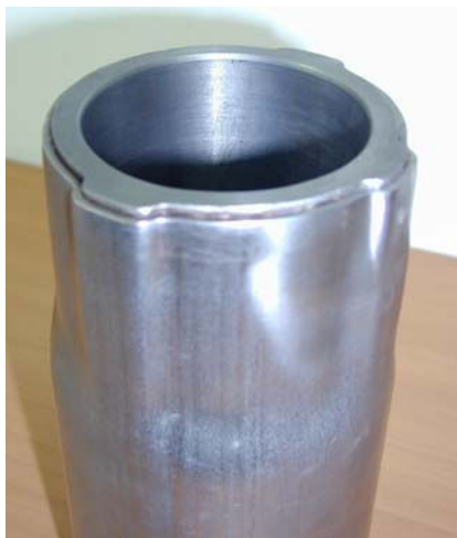
Figure 4: Tubular Forming 3 mm steel
