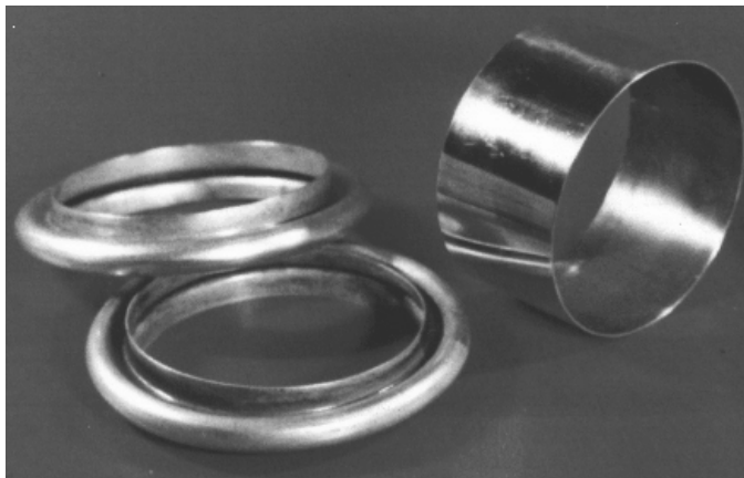
Figure 10: An equaliser of a torus form obtained from cylindrical billet
