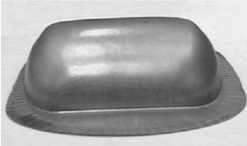
Figure 3: The reservoir from a material Dual-Stahl RVS 1.4462 stamped by explosion (size 280 x 380 mm; 1,8 mm thickness)
