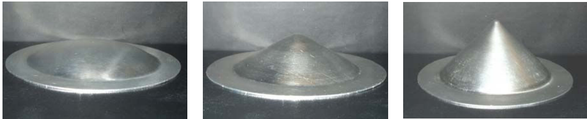
Figure 10: Promising examples produced by forming into a die without the rebound-effect
