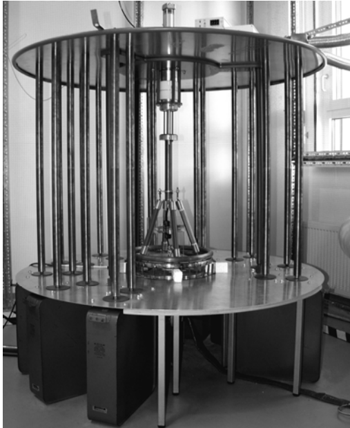
Figure 8: Coaxial 100 kA-impulse current generator with capacitive energy storage and without charging circuit
