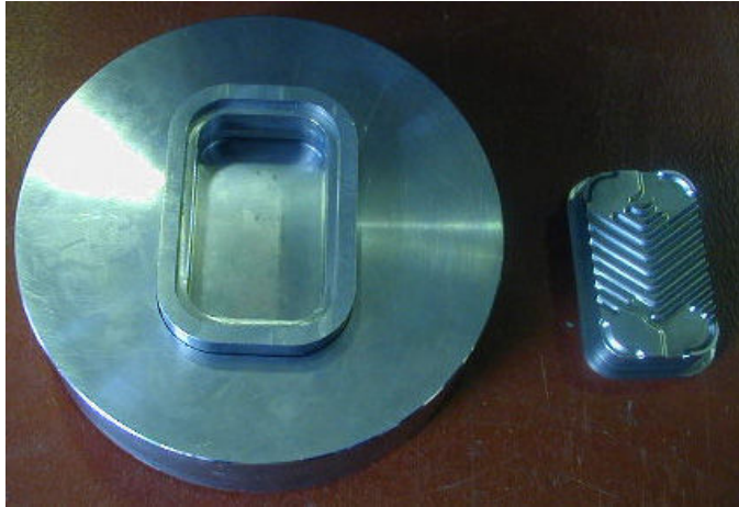
Figure 8: Forming Die Assembly Device
