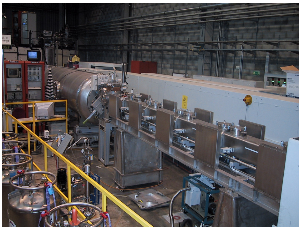
Figure 4.7: A SANS II instrument used for the small angle neutron scattering measurements at the Spallation Neutron Source (SINQ) at the Paul Scherrer Institut (PSI), Villigen, Switzerland.
