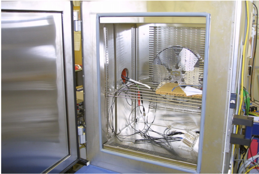
Figure 3.28: Climate chamber with sealed cable openings, set-up for wire bonded test devices and sensor for temperature logging
