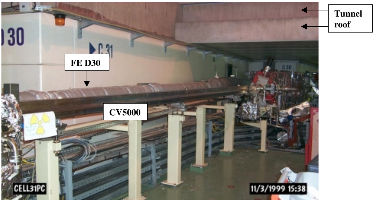
Figure 2-9 Photo of 8 mm inner aperture CV5000 vacuum chamber in ID31
