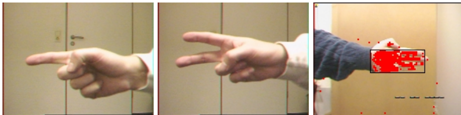
Figure 3.3: Examples of static hand gestures and, in the right image, the result of hand segmentation for hand tracking.
