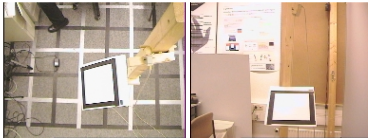
Figure 5.11: The corners of a rectangular plate are used as test points for investigation of accuracy of calibration. The left image shows a view from the ceiling camera, the right image a view from the side camera of our interaction environment.
