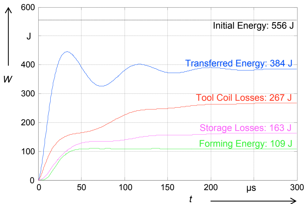
Figure 6: Variation of the different kinds of energy over time determined by the numerical field calculations for a forming process with a capacitor bank of 505 \mu\text{F} and an initial energy of 556 \text{ J} .
