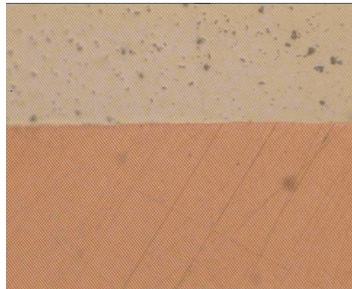
Figure 14: Al/Cu unetched x500
