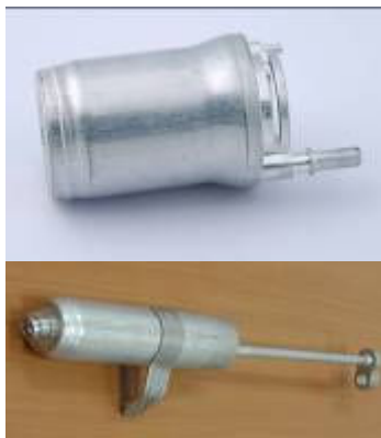
Figure 29: Al fuel filter and A/C receiver dryer
