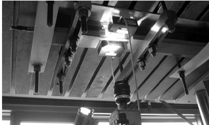
Figure 5: Cable-under-test clamped to the mounting plate, illuminated with a cold-light lamp, and observed with a high-speed video camera.
