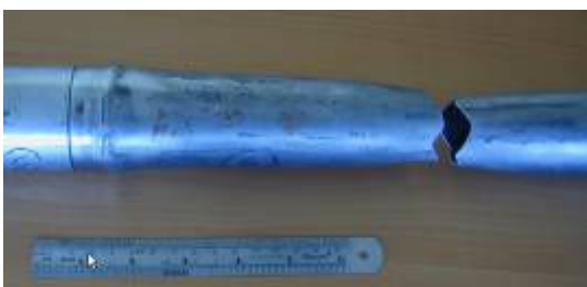
Figure 20: Tensile Test of welded 1020 steel tube
