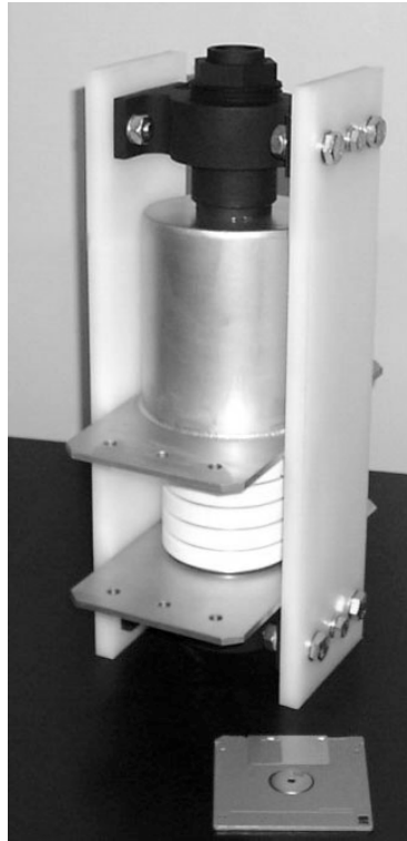
Figure 10: 200kA 12 kV RSD based switch with coaxial saturated core choke. di/dt=30kA/\mu s
