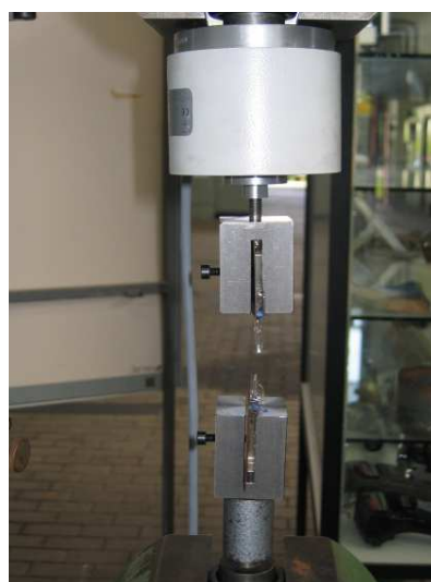
Fig. 4.8 Casting mould for tensile strength measurement and set-up of pull off test
