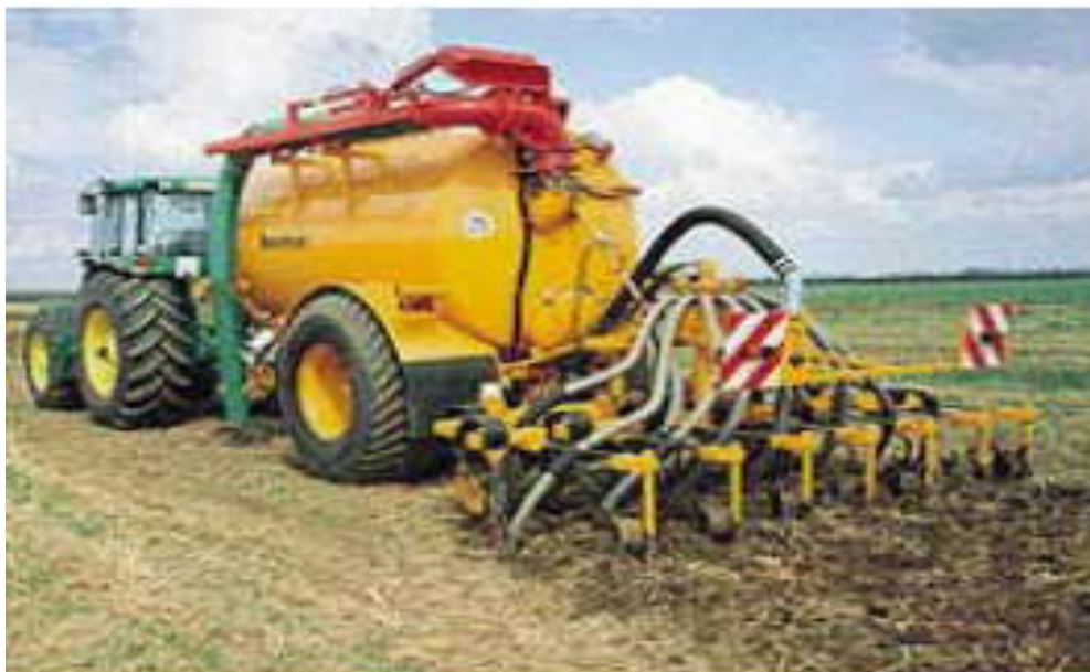
Figure 5-12 Urine fertilizer applied with mechanical injection (GTZ, 2005)
