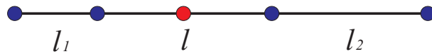
Figure 2.2: Ratio of boundary segment to its neighboring segments has to be checked, before merging.
