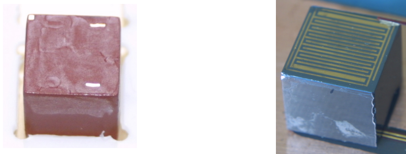
Figure 3.5: Left: Typical CPG detector by eV Products with red polymer-based passivation coating. Right: Naked detector used for TCT measurements [Oeh04]; the generation 3 CPG-electrodes can be clearly recognised.
