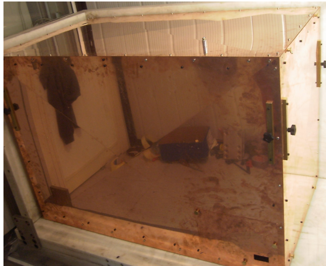
Figure 4.4: Photograph of COBRA's second Faraday cage. The screws used to fix the 1 mm thick copper onto the brass frame are visible. The small hole in the lower right corner of the side door is the cable channel.
