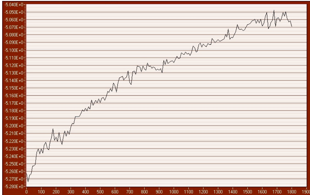
Figure 3.11: Plot of the leakage current between cathode and anodes (range: -5.28 nA to -5.04 nA) at 500V bias voltage vs. time (range: 0 to 1900 seconds). The moderate and apparently asymptotic decrease of the leakage current from its initial value at -5.27 nA to -5.06 nA after about 30 minutes is characteristic for CdZnTe detectors. The plot is displayed as exemplary measurement and was done with a 'reference'-detector (631972_07).
