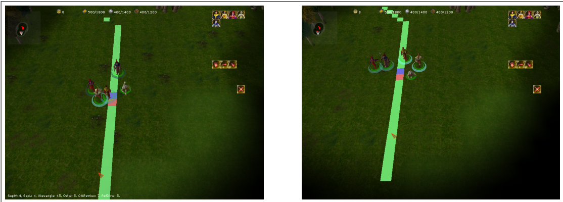
Figure 27: Parameters of the left picture: SeparationWeight = 4 ; SeparationDistance = 4 ; ViewAngle = 45 . Parameters of the right picture: SeparationWeight = 4 ; SeparationDistance = 4 ; ViewAngle = 180 . The angle of view of the units causes a different move behaviour of the group. In the left picture the smaller ViewAngle value causes that the group hangs together and each unit follows its unit in front. In the right one the group shows a more scattered behaviour because of the bigger ViewAngle value.
