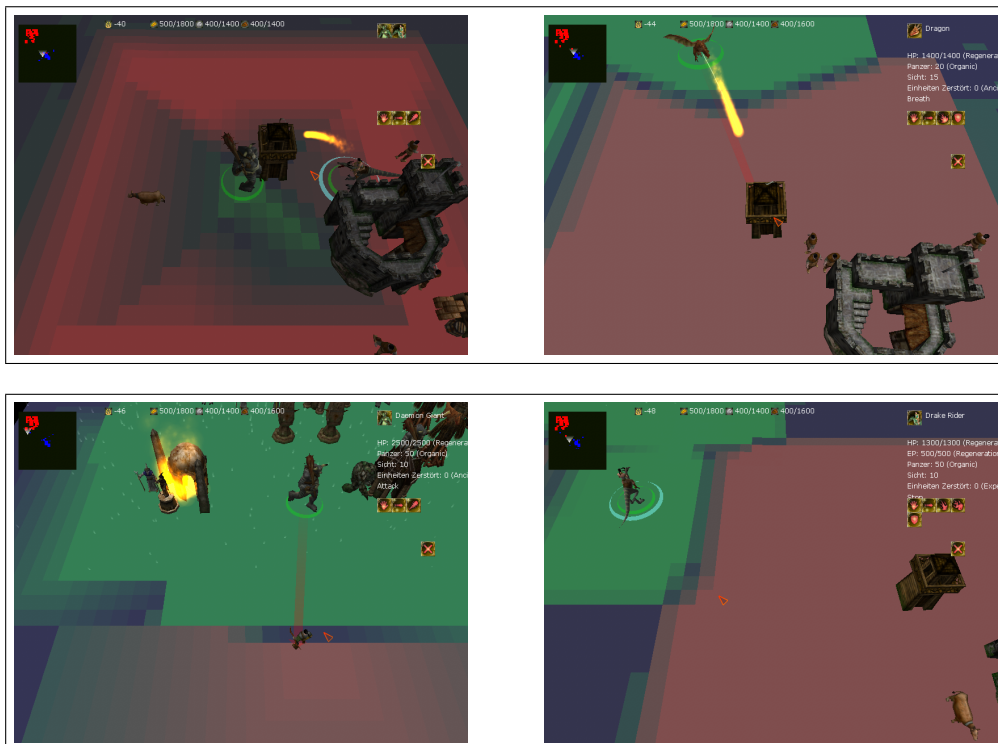
Figure 17: Activated IM visualization in four situations. The calculated influence values are transformed to colour codes and used to colour the ingame map cells. One can easily differ his own influence domain (green), the enemies influence domain (red) and the influence free areas (grey).
