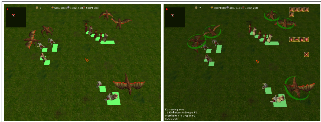
Figure 18: Screenshot of the SOM based selection. The left picture shows a group of friendly units, loosely gathered. The right picture shows a selected group of dragons (encircled) calculated by the SOM. You can see the debug information in the left-hand corner of the screen.
