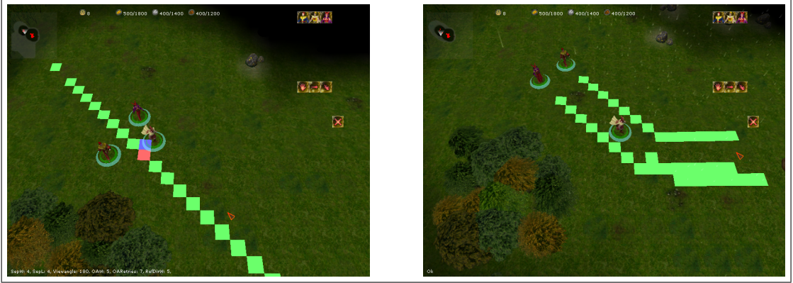
Figure 26: The left picture illustrates the visualization of the flock path. The path of the flock is highlighted in green, the average cell position of the group is pointed out in a blue coloured cell and the cell of the current path segment is coloured in red. The picture on the right shows the standard pathfinding, which calculates a different path for each unit of the group.
