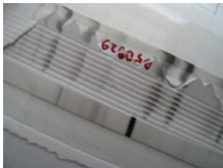
Figure 2.19: Photo of a laser ablated Indian ink stained membrane.
