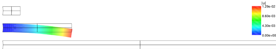
Figure 3.1: Three beam configurations BEAM-LH[2,8,32]-ANISO. Deformed state of the second beam, \|\mathbf{u}\| displayed. Prescribed analytical solution \mathbf{v} = (x_1 x_2, -\frac{1}{2} x_1^2)^\top , material steel.
