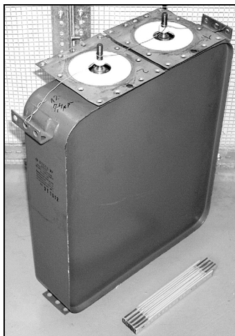
Figure 4: Impulse capacitor with C_N = 7,47 \text{ }\mu\text{F}
