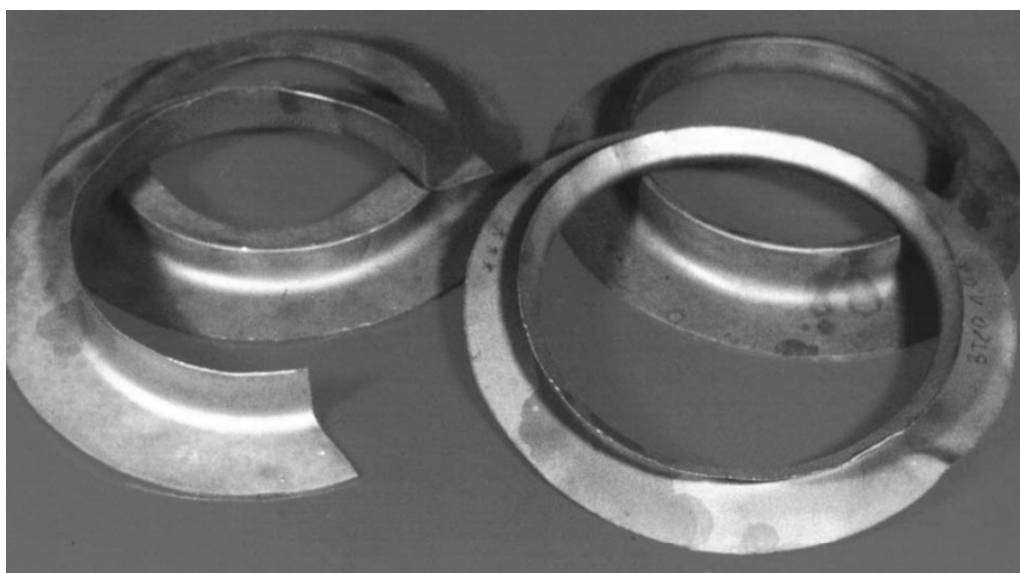
Figure 11: Details from low-deformable alloy stamped in a hot condition by explosion
