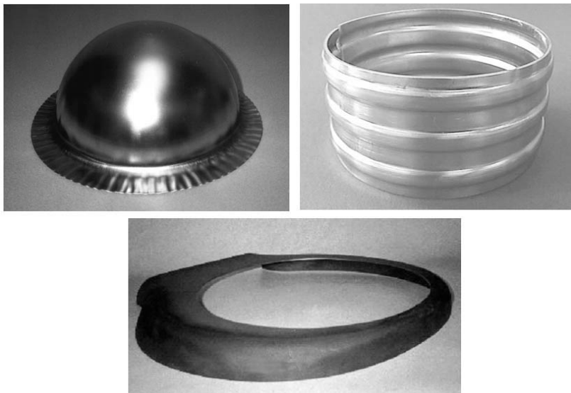
Figure 9: Details made by explosive forming
