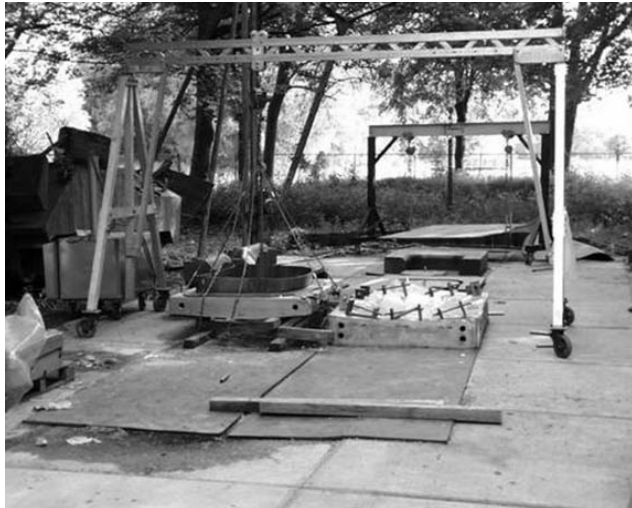
Figure 6: Stationary pool for explosion forming
