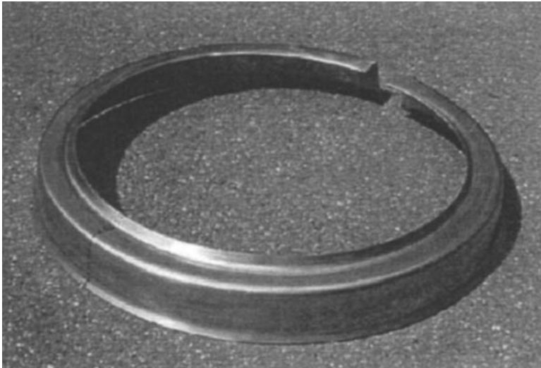
Figure 7: A ring frame from a material A2024 T3
