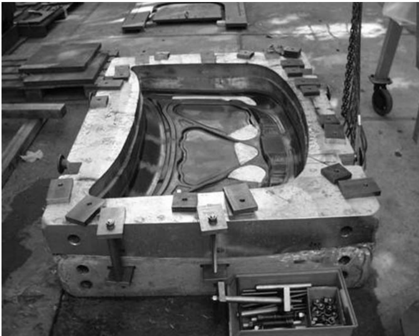
Figure 8: An equipment for explosion forming with technological inserts from plasticines
