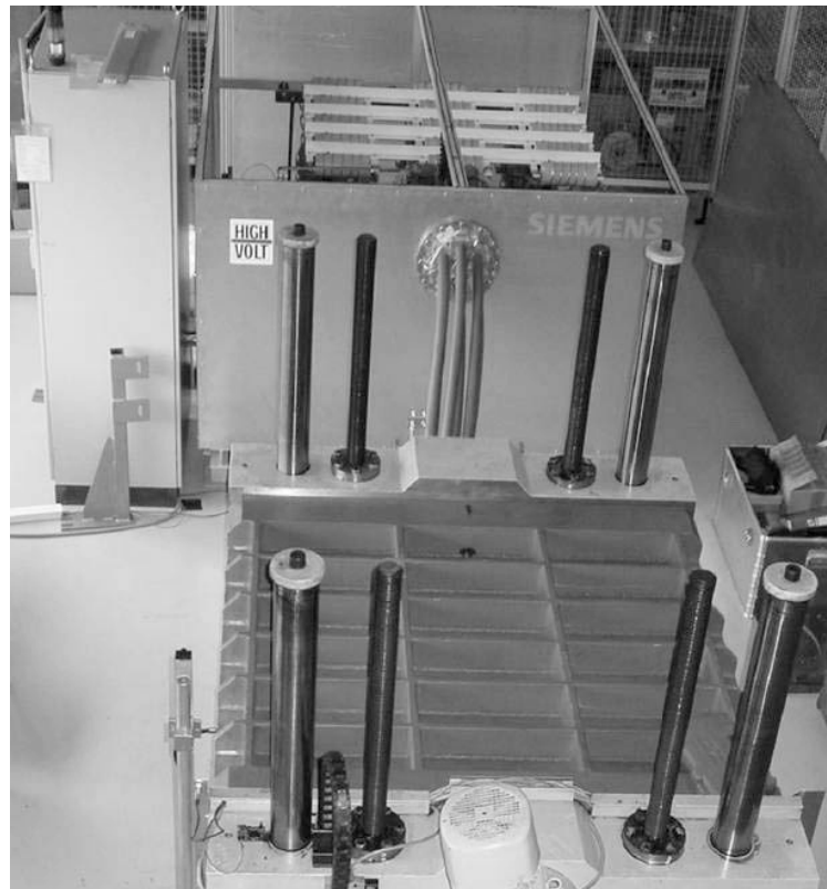
Figure 1: Photograph of the pulse generator installed at the FhG IWU, Chemnitz, Germany. In the foreground the workstation with the vertically moveable mounting plate for the experiment can be seen.
