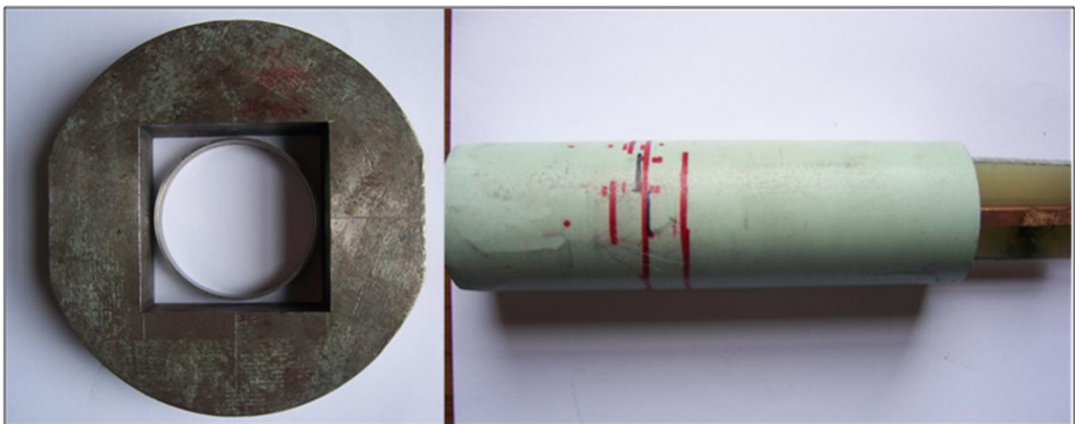
Figure 4: Experimental setup of electromagnetic ring expansion (a) Square die (b) Helical coil
