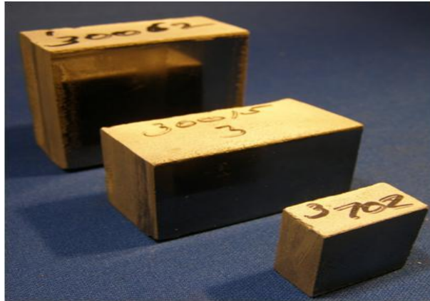
Figure 10: Typical shapes of the silicon carbide parts produced via axial DMC process
