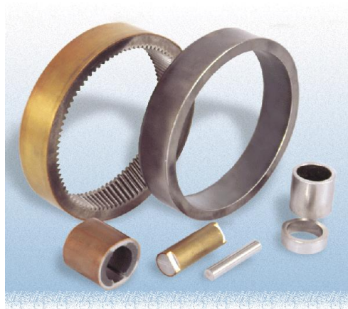
Figure 9: Typical shapes of the parts produced via radial DMC process
