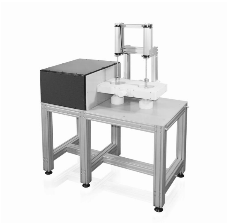
Figure 6: Multiple joining coil for parallel processing of two work pieces (MJo2).
