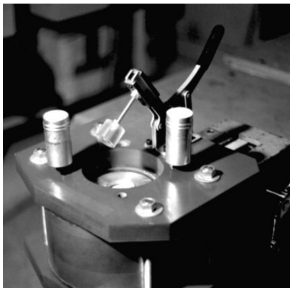
Figure 13: Typical EMF Systems as used in the Aerospace Industry for the assembly of Flight Control Tubes shown in Figure 12
