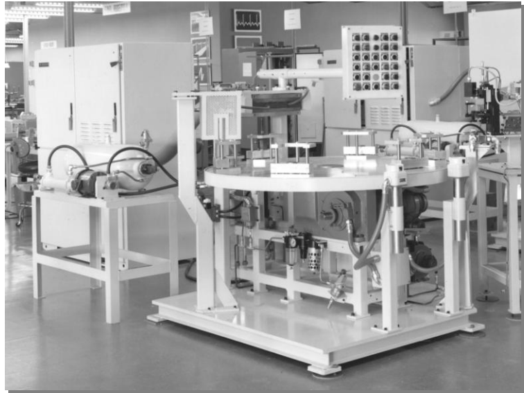
Figure 17: EMF systems with automated turntables to assemble worm gear components for automotive power steering.
