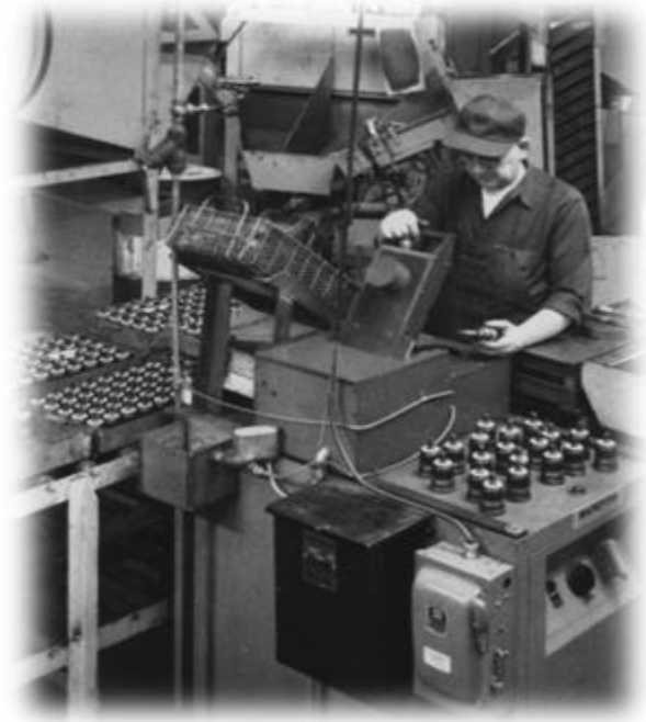
Figure 3: First industrial application used to shrink retaining rings onto neoprene boots. The above picture shows the ball joint before and after assembly.
