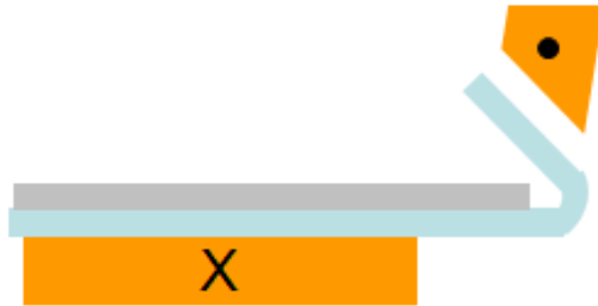
Figure 5 Pre-flange actuator with workpieces. The inbound and outbound currents were labeled onto the actuator. (The supporting blank holders are ignored in this figure.)
