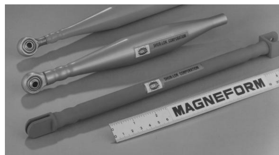
Figure 9: Aircraft Control Rod (Electromagnetic Compression Operation). The tubes have been anodized prior to forming. There is no surface damage to the anodized finish.
