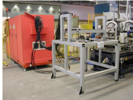
Figure 7: EMF stand incorporating a coil that releases forming energy to moving workpiece (right)
