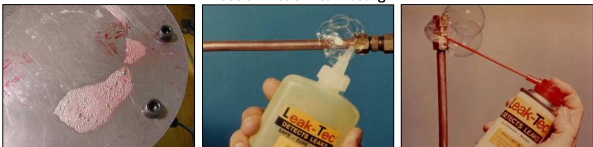
Figure 114 BELT using various bubble-forming solutions on different machinery elements [WS8], [WS35]
