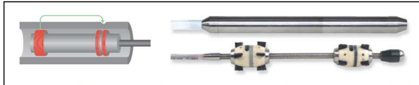
Figure E8 A picture representing the conceptual design and two actual probes used in RFT testing. The upper one is dual exciter used for inspection of tubes and the lower one is specifically designed for inspection of boilers (Adapted and retrieved from www.olympusndt.com in February 2008).
