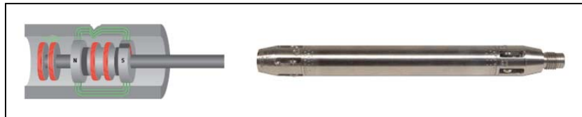
Figure E6 A picture representing the conceptual design and an actual probe used in MFL testing [WS71]
