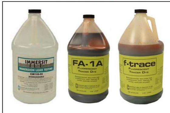
Figure 122 Different liquid sensitivity improvers for HSLT. From left to right: surface tension reducer liquid; water soluble and florescent tracer liquid [WS8]
