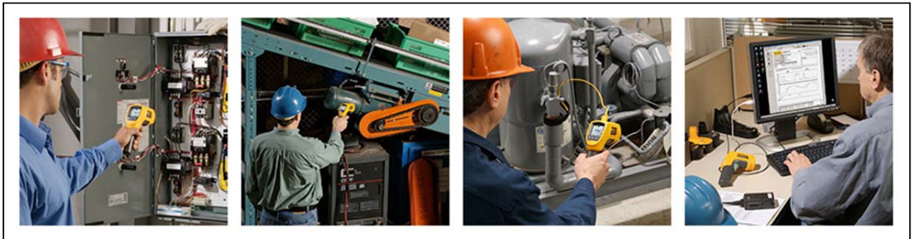
Figure E21 Different applications of thermal inspection. From left to right: Electrical - to check electrical panels, wiring and cables, ballasts, transformers, motors and etc.; Mechanical - to check hydraulics, gears, shafts, bearings, pumps and etc.; Facility - to check duct leakage, liquid flow in pipes, roofs, valves, steam traps and etc.; Condition Monitoring and Trending [WS2]
