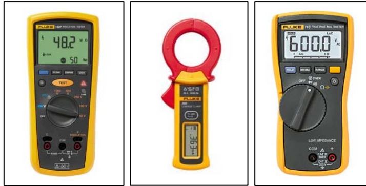
Figure 91 From left to right: a digital Megohm-meter, a clamp current-meter and a digital multimeter [WS3]
