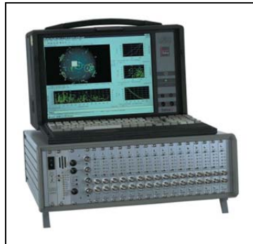
Figure E1 A multi-channel system for acoustic emission detection and analysis [WS102].
