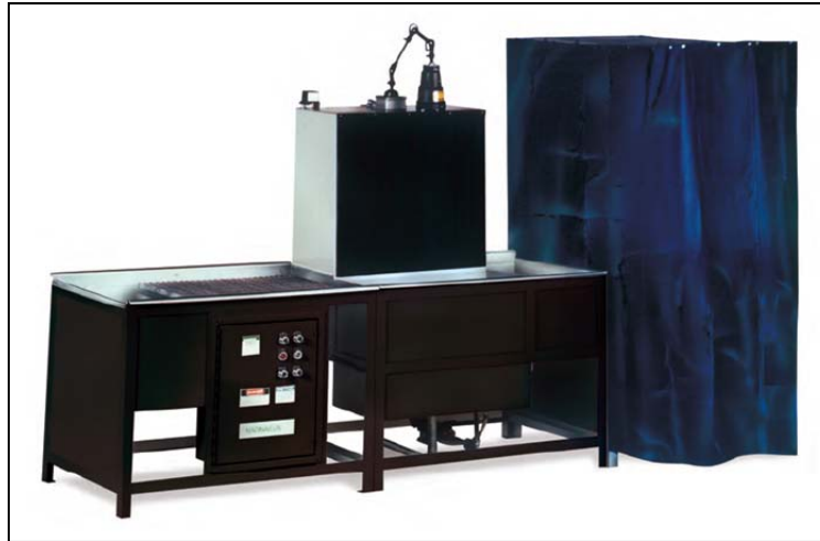
Figure E16 A PT stationary unit designed for water washable method with six different stations: penetrant station, drain station, wash station, dryer station, developer station and inspection station [WS62]
