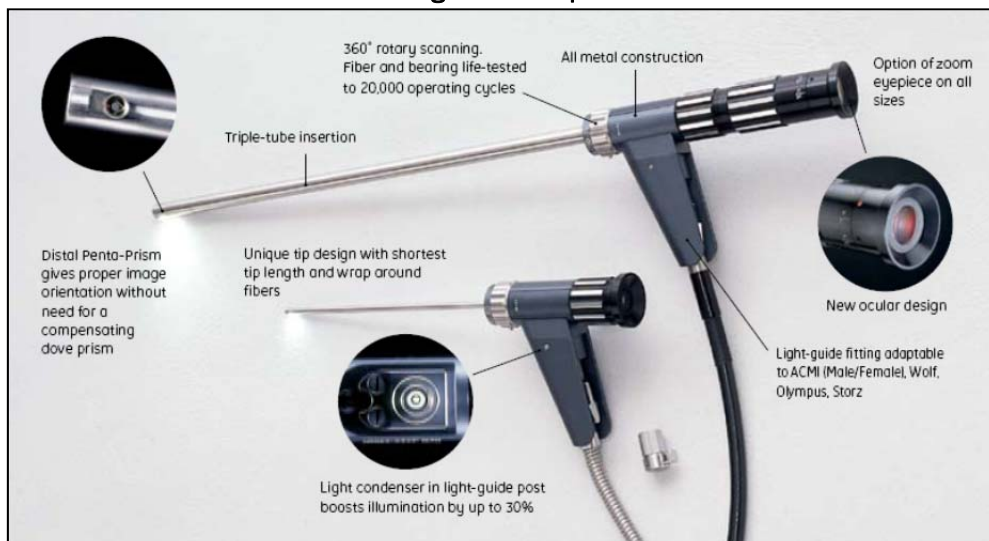
Figure E28 A rigid borescope with brief information of its different components [WS44]
