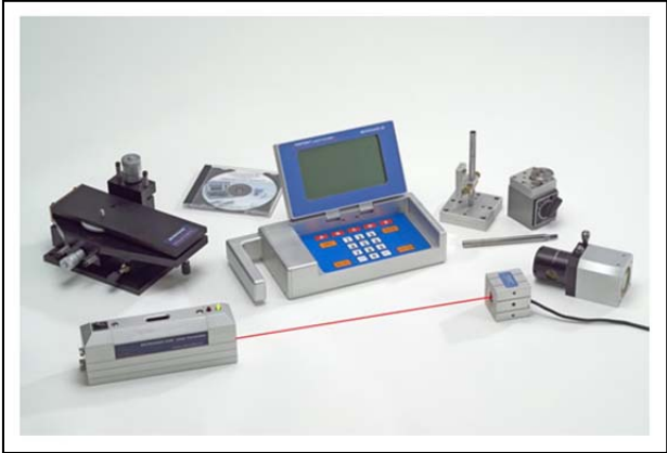
Figure 110 A laser microgage system consisted of a LMG transmitter and receiver plus a digital processor [WS77]
