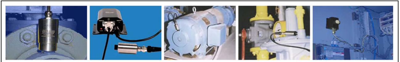
Figure E25 A variety of tools and monitoring applications of online continuous UT. Ultrasonic sensory systems provide information about valve leakage, bearing and lubrication condition, flow disruption, and monitoring of electronic cabinet for arcing [WS100]
