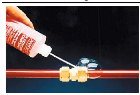
Figure E11 A gas leak detection solution [WS28]
