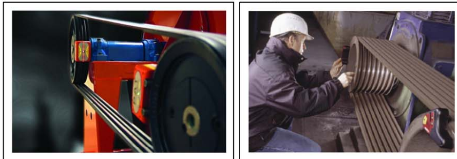
Figure 107 Laser belt alignment systems with laser transmitters that fit into the pulley grooves [WS38], [WS84]
