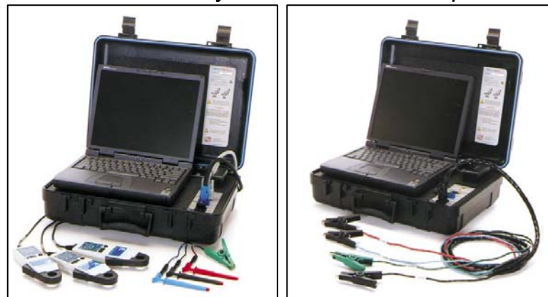
Figure E4 Photos of E MAX dynamic inspection device (left) and MCE static inspection device (right) [WS74]
