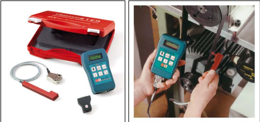
Figure 111 A trummeter used to precisely measure and correct belt tension on a motionless belt [WS48]
