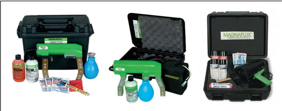
Figure E14 Three different portable MT kits. From left to right: Magnetizing yoke kit used for dry particle inspection, similar kit with battery powered yoke, and dry particle inspection kit with black light which requires a magnetizing yoke in addition [WS61]
