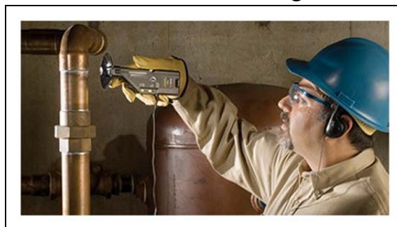
Figure 131 Use of a handheld ultrasonic device to detect leaks in piping [WS59]
