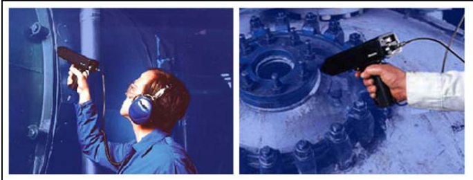
Figure E22 Two different analog UT instruments. From left to right: an advance instrument used for contact and airborne applications with frequency tuning and meter mode, a simpler tool for airborne leak detection and mechanical inspection [WS100]
