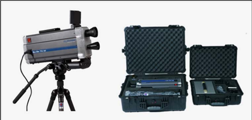
Figure 112 A carbon-dioxide laser camera for identification of hexafluoride gas leaks [WS101]
