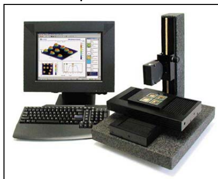
Figure 102 A desktop laser profilometer for inspection of small objects [WS87]
