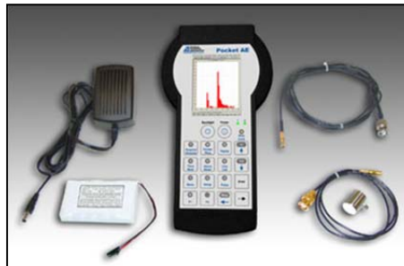
Figure E2 A hand-held instrument and some sensors for AE measurement and leak detection [WS73]
