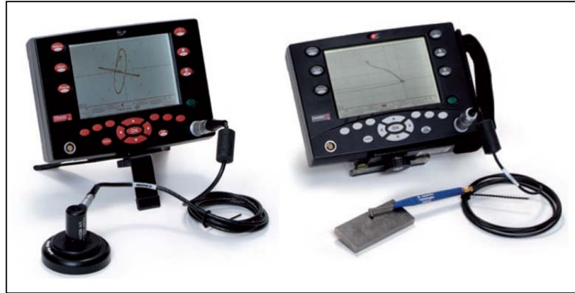
Figure E5 An image representing different portable EC tools. From left to right: a dual frequency EC instrument for crack and corrosion detection, a single frequency EC tool for crack and corrosion detection with conductivity and coating measurement [WS44]
