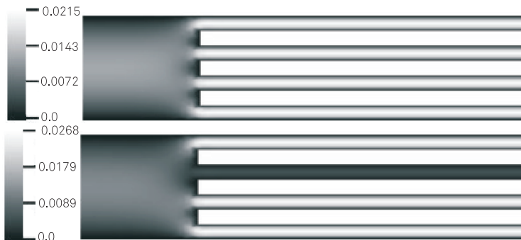
Figure 6.3: The Euclidean norm of velocity. Top: The flow is not blocked. Bottom: The flow at the second channel is blocked
