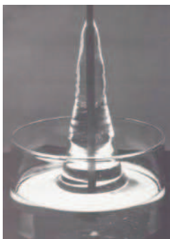
Figure 1.4: The rod climbing effect [11]. Permission from Elsevier and Prof. David V. Boger.
