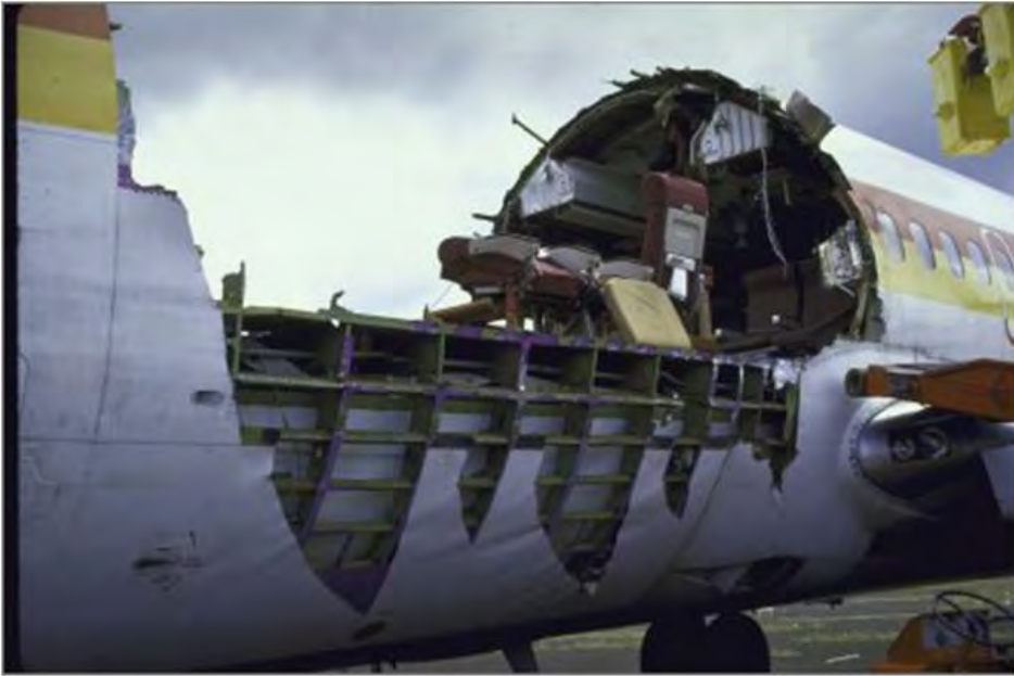
Figure 3.1: The severely damaged fuselage of the Aloha Airlines Boeing 737, following the accident on April 28, 1988
