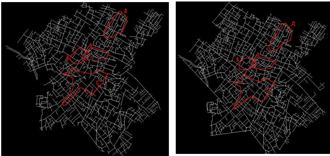
Fig. 7-18: The axial map of Yazd before the construction of new streets in 1940s (left) and after the construction of the streets (right). Four areas that are analyzed by Space Syntax Theory; A: Fahadan neighborhood, B: Do-Menar neighborhood, C: bazaar, and D: city center and the area around the Jame mosque of the city.
