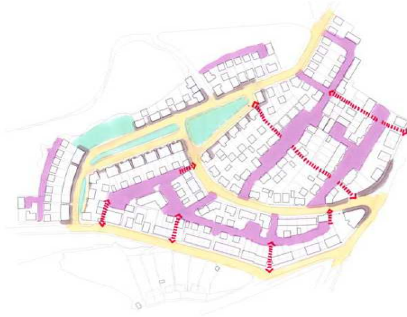
Fig. 3-11: The hierarchy of the streets and routes of Coed Darcy according to its master plan.
