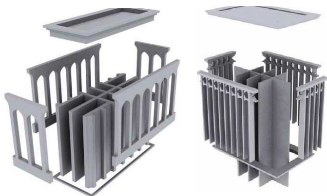
Fig. 5-15: Illustration of the elements of the body of Badgirs; the panels, the inner blades, and the ceiling are seen in these images (Roaf, 1988)
