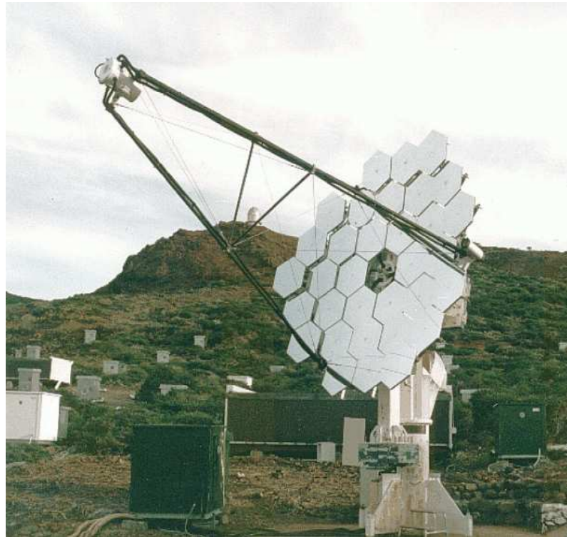
Figure 4.4: The HEGRA telescope CT 1 after the upgrade with hexagonal aluminum mirrors in 1998 [K + 98].
