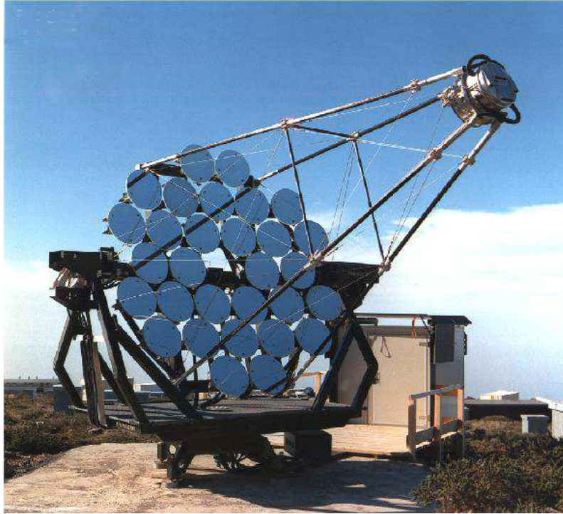
Figure 4.5: The HEGRA telescope CT3 of the HEGRA Cherenkov telescope system [Ast07].
