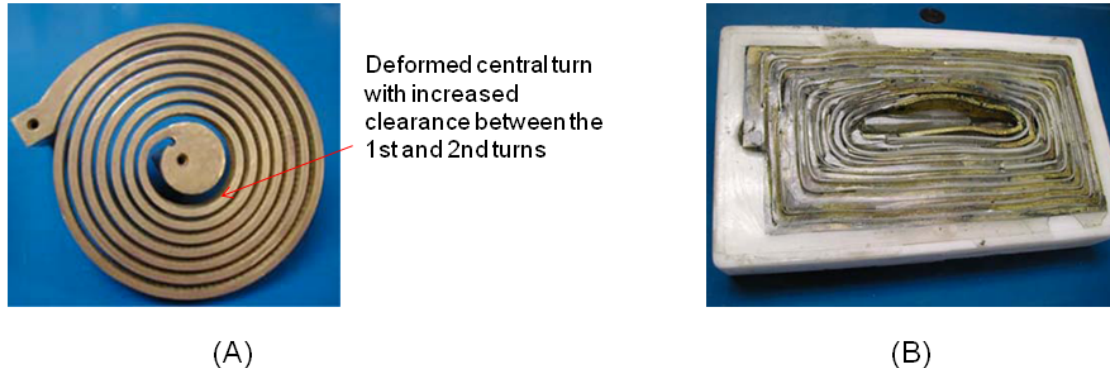
Figure 1. (A) The spiral of a circular flat coil with deformed 1 st and 2 nd turn, (B) Coil fractured due to the deformation of the central turn [2]
