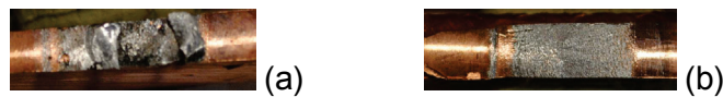
Figure 11: Typical fracture surface of Al/Cu weld - (a): relatively good weld, (b): weld with intermetallic phase
