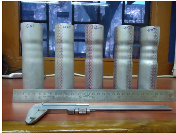
Figure 2: Electromagnetically deformed tube specimen at various energy levels
