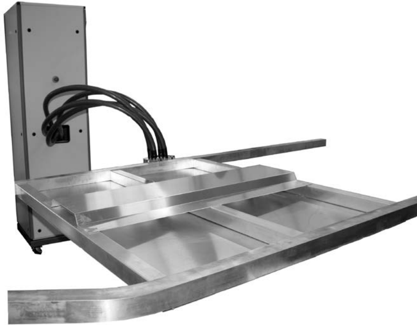
Figure 6: EMPT welding of larger subassemblies
