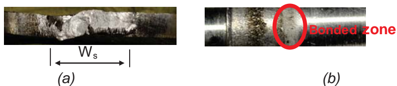
Figure 3: Illustration of a fracture surface with residue (a) or without residue (b)
