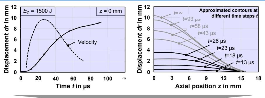
Nearly parallel expansion of the tube wall ( $z \approx 0 - 6$  mm)
