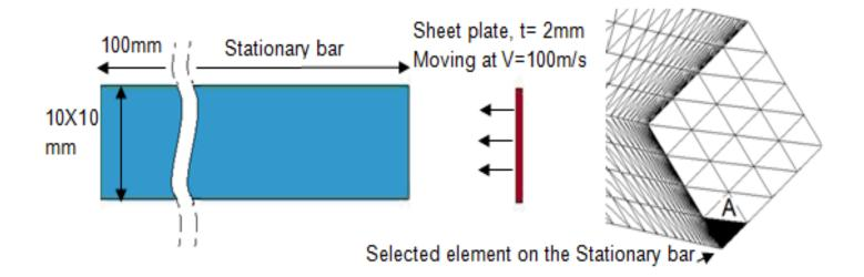
Unphysical peak in contact pressure in element A of the impacted bar
