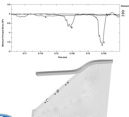
Theoretically, the ideal mesh should be uniform in all directions and get convergence for the critical values of the problem. However, it should be fine enough to give accurate results so that further refinement dramatically runs up the cost of computing with negligible improvement in accuracy
