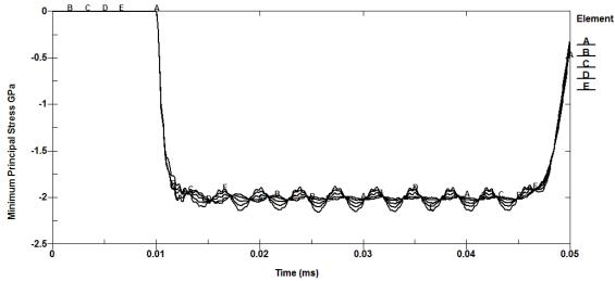
bulk viscosity TYPE 1 was used with coefficients Q1= 1.5, Q2= 0.06. Soft= 1 penalty formulation was used that takes into account the nodal masses and global time step size in contact stiffness calculations to achieve better stability.
