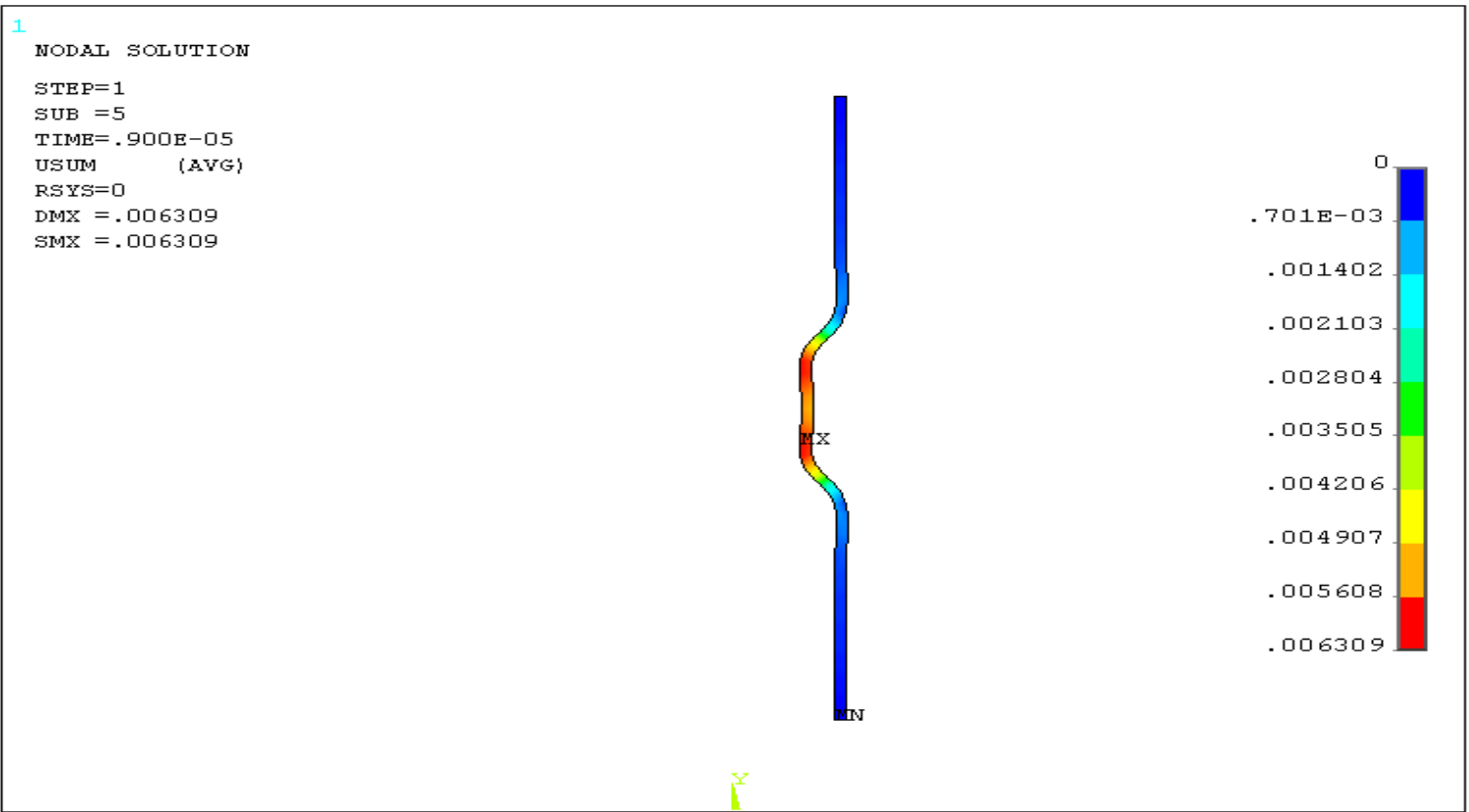
Figure.8 . The sectional view of the deformed tube for an energy level of 18 kJ at 9 \mu s
