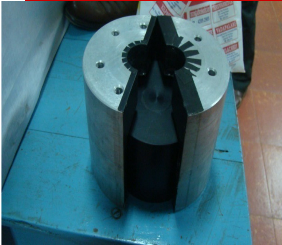
Fig.2 Field shaper in the experimental set up
