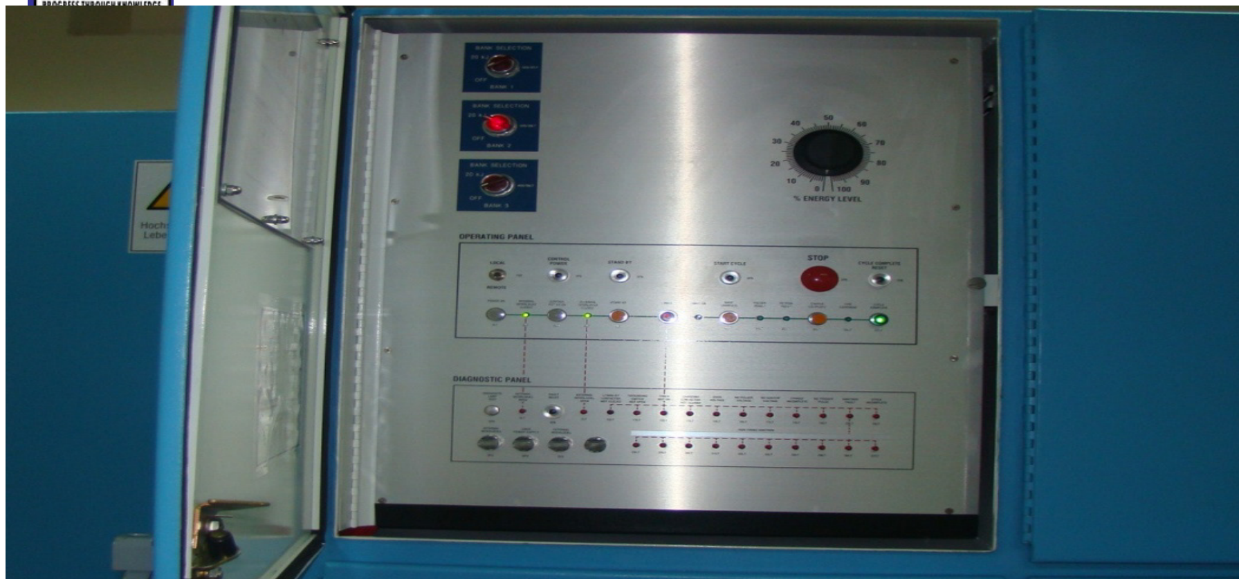
Fig.4 Experimental configuration showing the bank selection, % Energy level, Operating panel and Diagnostic panel.
