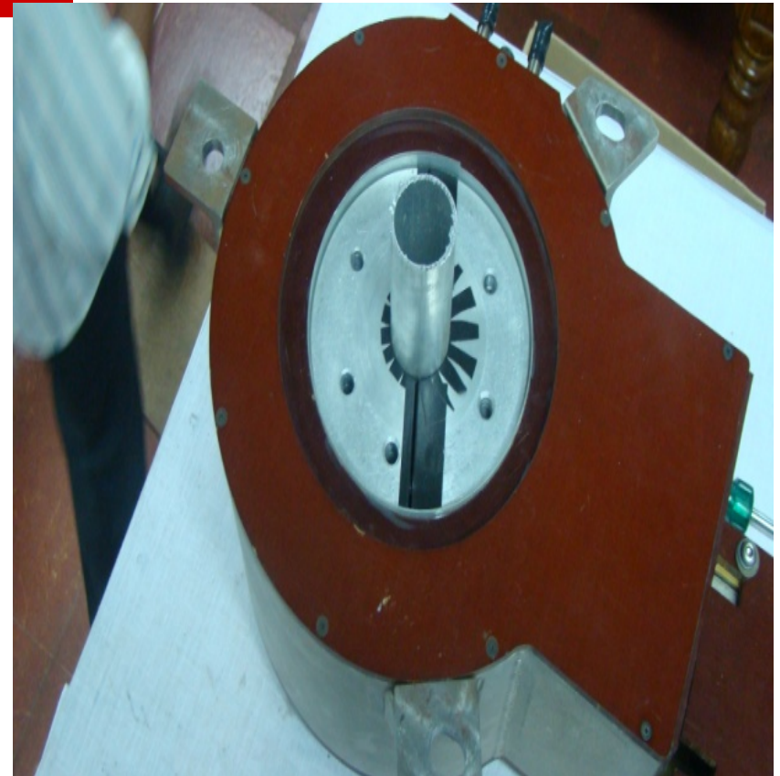
Fig.2 Field shaper in the experimental set up
