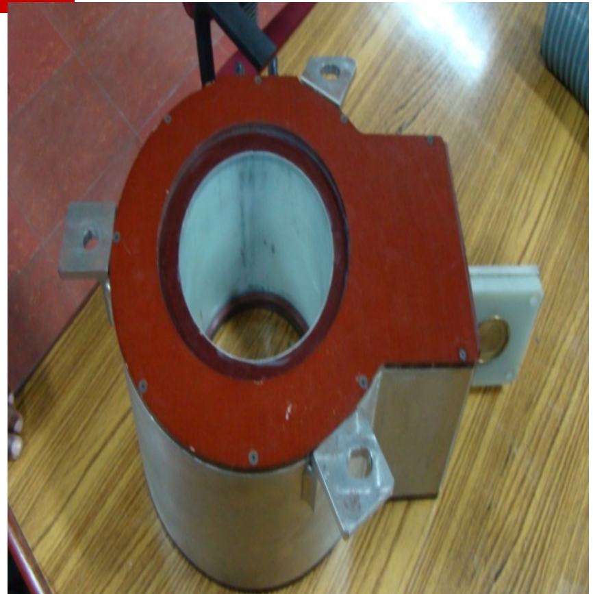
Fig.1 Photographs of the 4-turn solenoid coil built by PST Products, GmbH.
