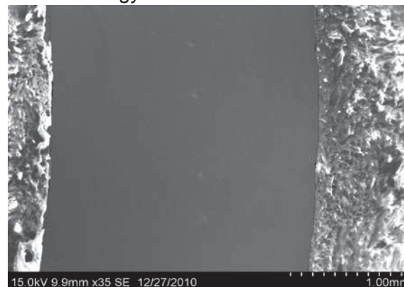
Figure 5: SEM micrograph of aluminum alloy specimen for measuring Vickers hardness
