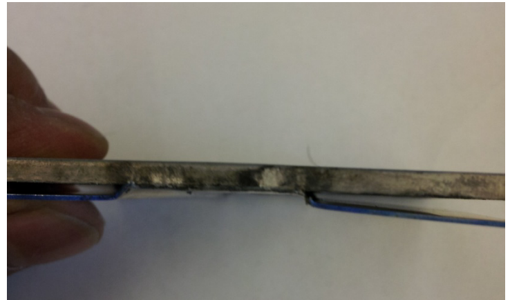
AA6061 T6 welded with AZ91D (mag alloy)
