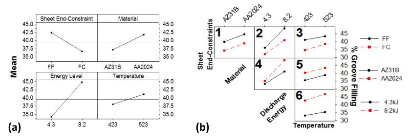
(a) Main effect plots, (b) Interaction plots, of all the factors taking maximum filled groove height/Total groove height as a response.
