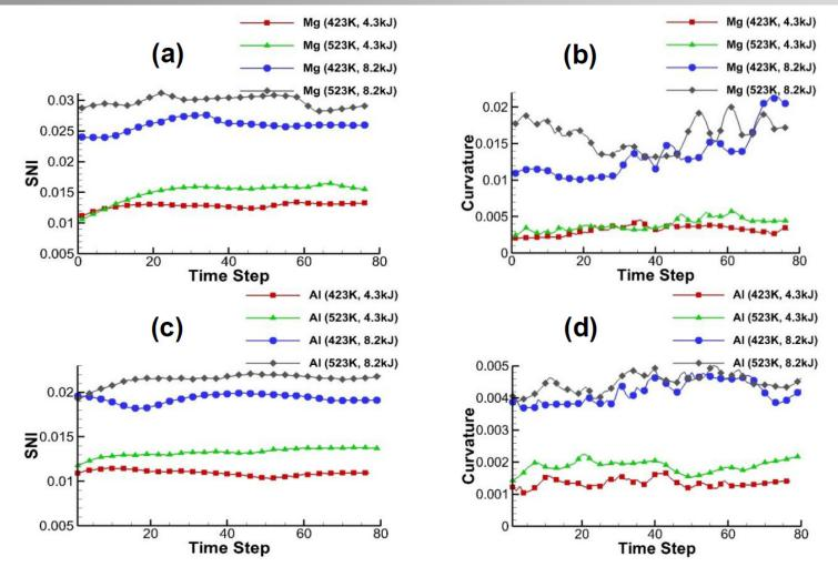
(a) & (c) SNI plots, (b) & (d) Curvature plots for runs with Mg-alloy & Al-alloy respectively for fully Clamped end condition.
