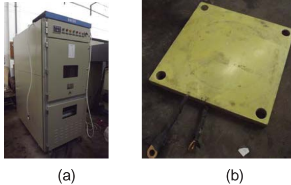
Fig.2 EMF equipment (a) Capacitor bank and vacuum switch (b) Working coil
