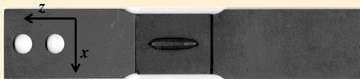
Specimen for pure-shear loading condition
