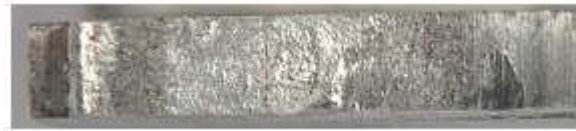
Beginning of bonding (trace of residue)
