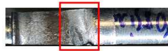
Beginning of good welding (thin weld)
