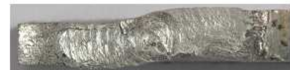
Beginning of good welding (thin weld)
