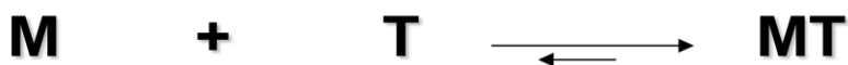
Figure 2.13 Stoichiometric Imprinting: strong interactions between Monomer (M) and template (T) lead to MIPs with increased capacity and affinity for the template.
