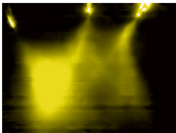
Figure 5.4 Photo of three electrosprays obtained from the multi-nozzle DB-ESI system operated at 3 kV with solution: methanol-water 1:1+1 % acetic acid + fluorescein. Exposure time 2 s.
