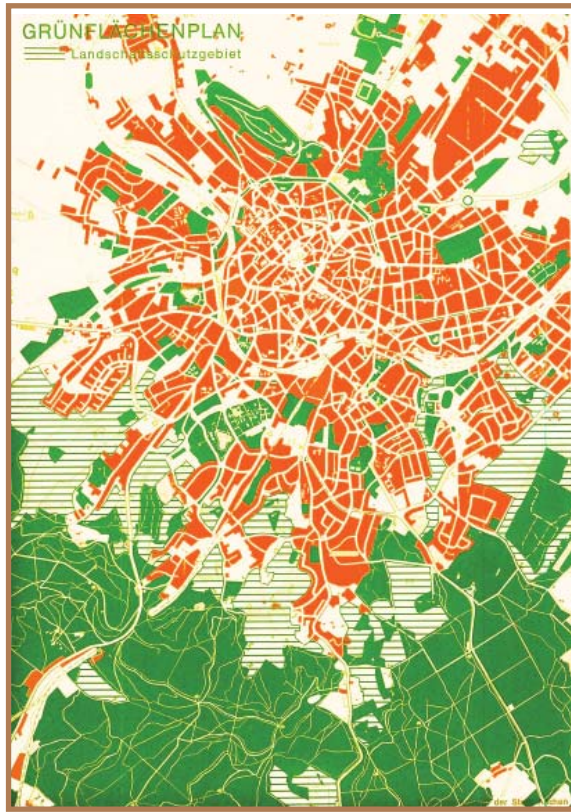
Plan 5 - Expansion of the Green Fingers according to the Second Development Planning of the City of Aachen, 1957. red = built forms white = access roads and hard surfaces hatched green = grassland green = tree and shrub Reference: Aachen - Eine Stadt an der Grenze baut auf. 1957.
