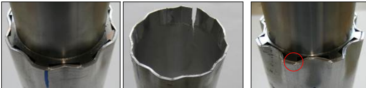
Figure 7: Close-up of the groove zone of a test specimen before (left) and after (right) torque testing
