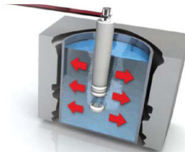
Figure 1: Electrohydraulic forming of a tube
