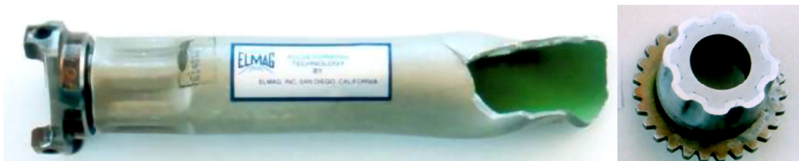
Figure 1: Magnetic pulse crimped torque joint used in the Boeing 737, 747 and 777 aircraft. Left: after torque testing [1]
