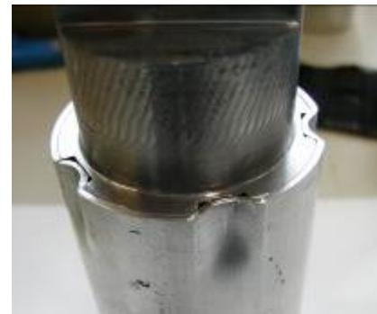
Figure 5: Example of a torque crimp connection (internal workpieces with 5 grooves)
