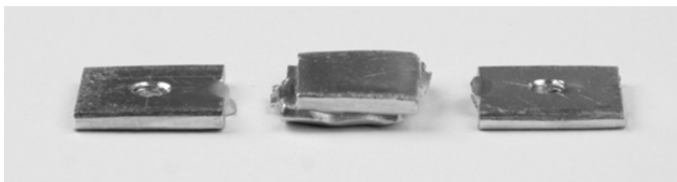
Figure 3: Welded specimens (center) with the clamped parts.
