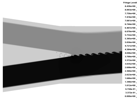
Figure 2: Example of wavy interface with jetting on LS-Dyna, density contours - Al / Steel
