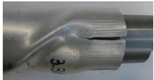
Figure 17: Failure mode 3: tube buckling, with cracking
