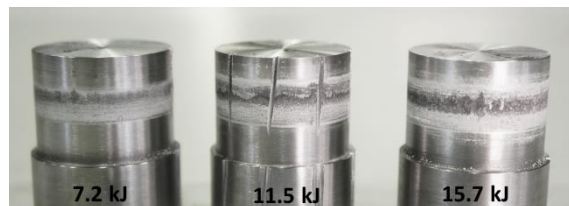
Figure 5: Samples with 10 mm working length at various energies.
