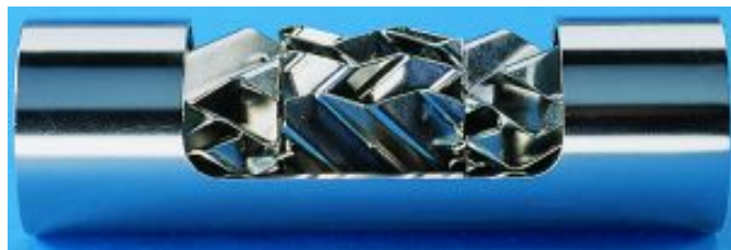
Figure 4.13: Laboratory scale Sulzer SMV TM static mixers, 3 adjacent mixer elements relatively rotated by 90°.
