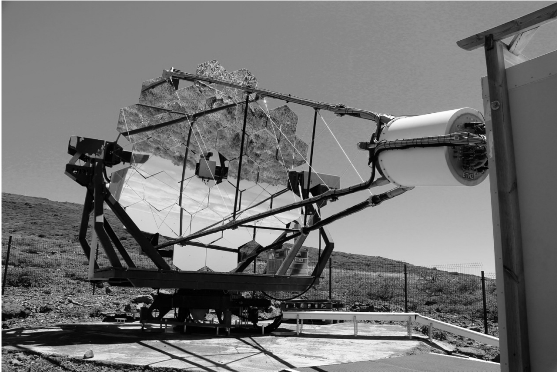
Figure 5: The FACT telescope. One can see the mirror plane and the camera embedded in the white metal cylinder. (MAGIC-Homepage, 2010).
