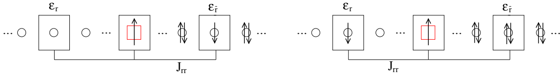
Figure 7.13: Part of the Hamiltonian H_r which consists of the sites on which it first becomes energetically favorable to remove a particle from the Fermi sea so that the spin-flip term can act on the respective site. Because of the particle-hole symmetry, removing a particle from a negative level results in the same energy loss as adding a particle to the corresponding positive level.
