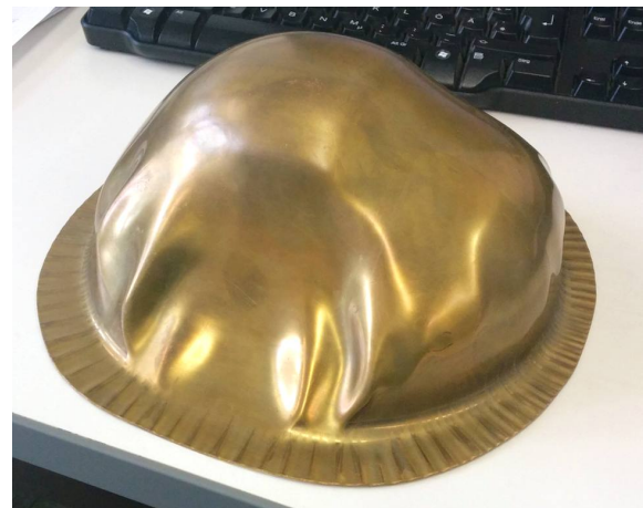
(b) Vacuum formed brass surface for use with force control tests.
