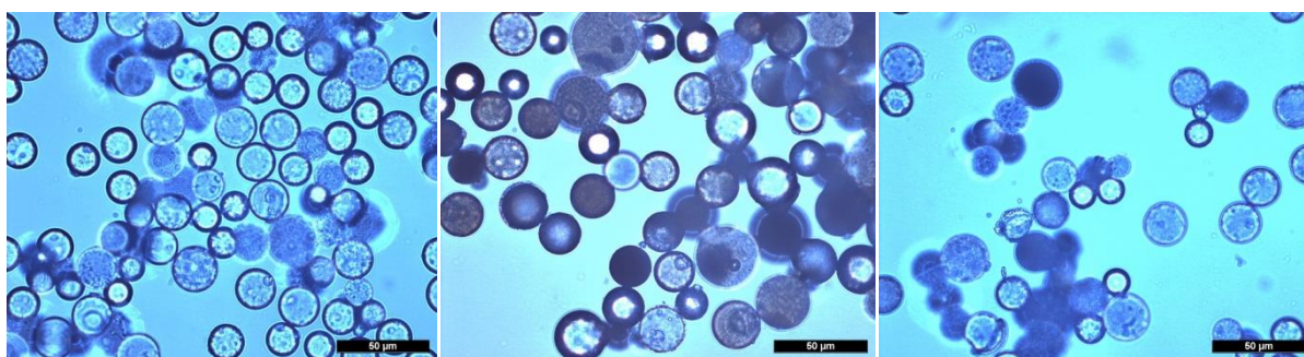
Figure 61 Displays pore-filling composite microscopy pictures: (left) bare silica (middle) silica with polymer and (right) polymer replica of the etched silica.
